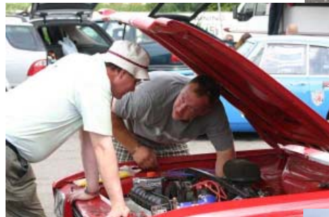
Simon Groves and Mike Hayward cable tying the plug leads in place after the Capri went onto five cylinders at Mallory.
